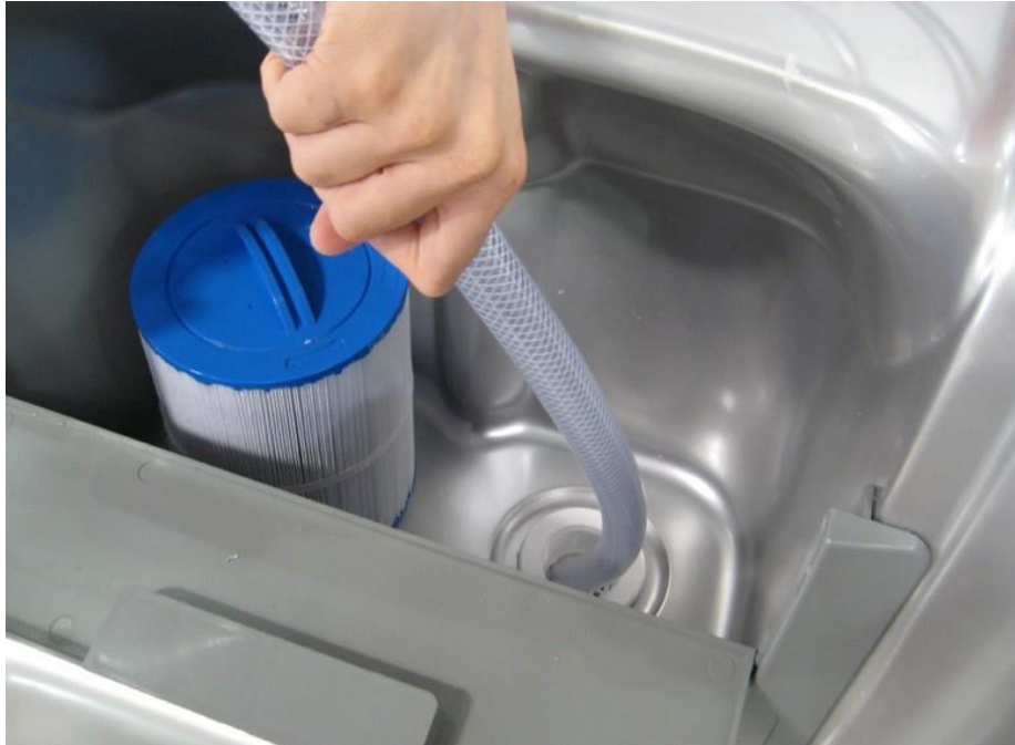
Figure 18. Filling Location in Filter Housing
